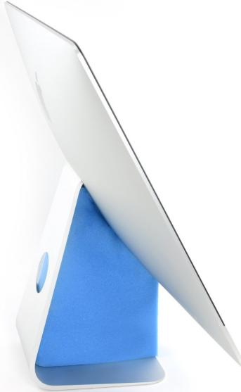
**i** With the hinge free to move, the iMac will be unbalanced and hard to work on. Repairs can be completed as shown, but are faster and easier with an [iMac service wedge](#).
